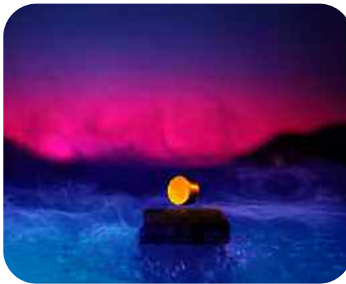
A magnet levitating above a superconductor cooled with liquid nitrogen – another example of an emergent phenomenon.
